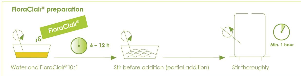
For better sedimentation Tannivin® Galléol and a bentonite suitable for beverage treatment can be added as reaction partner. The required FloraClair® amount for several working days can be prepared in advance since, under normal conditions, the plant protein has good microbiological stability.
